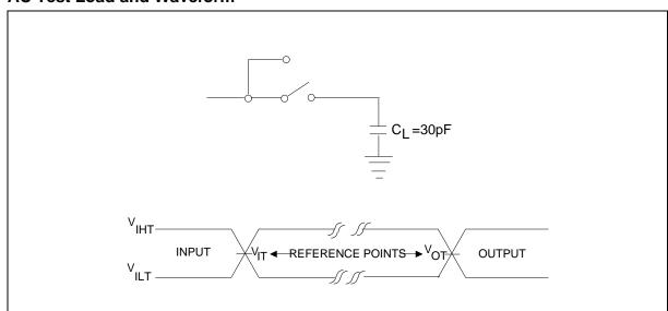
AC test inputs are driven at Viht (0.9 Vdd) for a logic "1" and Vilt (0.1 Vdd) for a logic "0". Measurement reference points for inputs and outputs are at Vit (0.5 Vdd) and Vot (0.5 Vdd) Input rise and fall times (10%  $\leftrightarrow$ 90%) are <5 nS.
